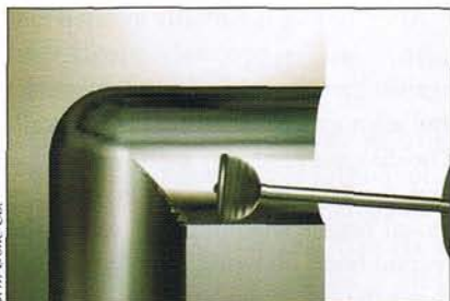
An in-line tool allows drilled cross-holes to be deburred without moving parts to another area of the shop.
