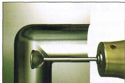
An in-line tool allows drilled cross-holes to be deburred without moving parts to another area of the shop.
