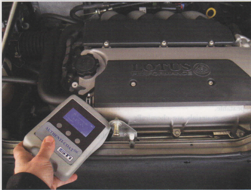
STI says that a measuring device could detect whether coatings for engine components are worn through, without having to disassemble the engine.
