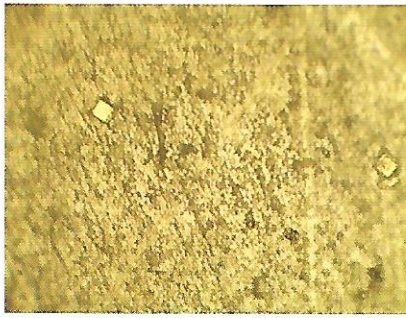
Image 5: A 400x view of the surface of a coating incorporating structured micro taggants to permit authentication of a product simply by microscopic examination
