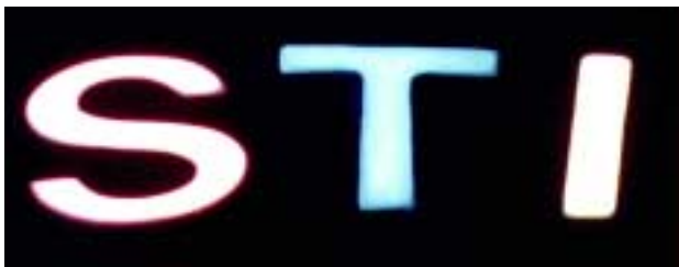
Photo 3 – Aluminum shapes coated with composite EN with three colors of light emitting particles photographed under UV light
