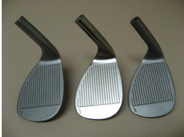
Photograph 2 – Three golf clubs coated with (left) a 0.001” thick under layer of high phosphorous electroless nickel followed by 0.001” thickness of a composite electroless nickel and diamond coating; (center) 0.001” thickness of a composite electroless nickel and diamond coating over coated with a 0.0002” thick layer of medium phosphorous electroless nickel; and (right) a single layer of 0.001” thickness of a composite electroless nickel and diamond coating
