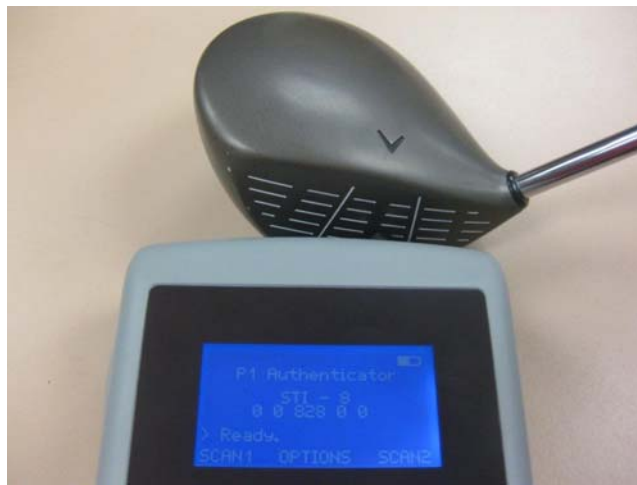
Photograph 2 – A detector displaying the presence of material “STI-8” in the coating on a golf club, one example of the products that can be enhanced with this composite identification technology.
