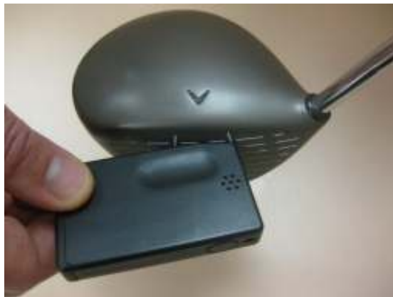
Photograph 3 – This extremely small detector makes a distinct sound when in contact with a specialty coating.
